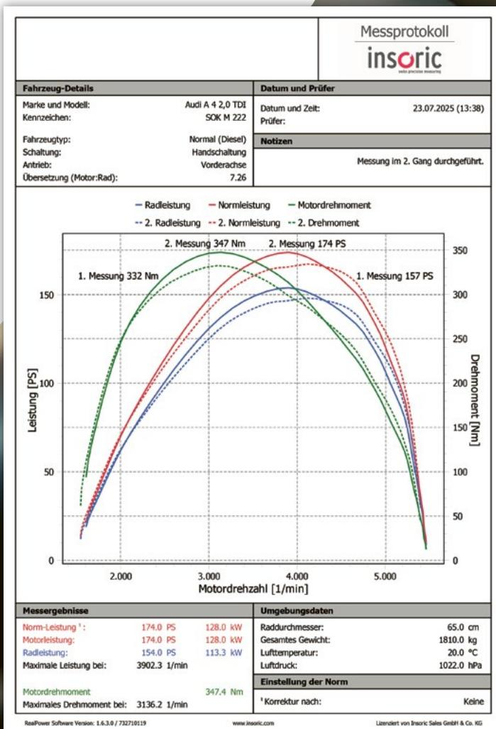
The first measurement was taken on July 22 (dashed line). 300 ml of our **HIGTEC PREMIUM CLEANER DIESEL** (Art.-No.: 23063) was then added to the fuel tank and the tank filled up completely.
