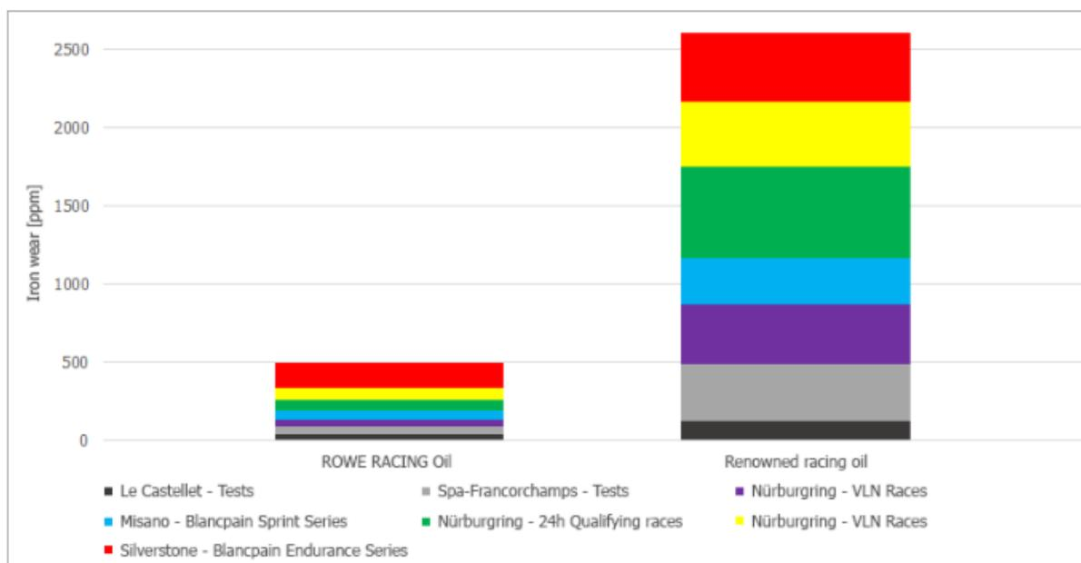
The diagram (above) shows the iron wear accumulated over several races/test drives. The iron already shows more wear with the renowned racing oil after the third run (right) than it does with the ROWE RACING oil (left) after all 7 races / test drives together.
