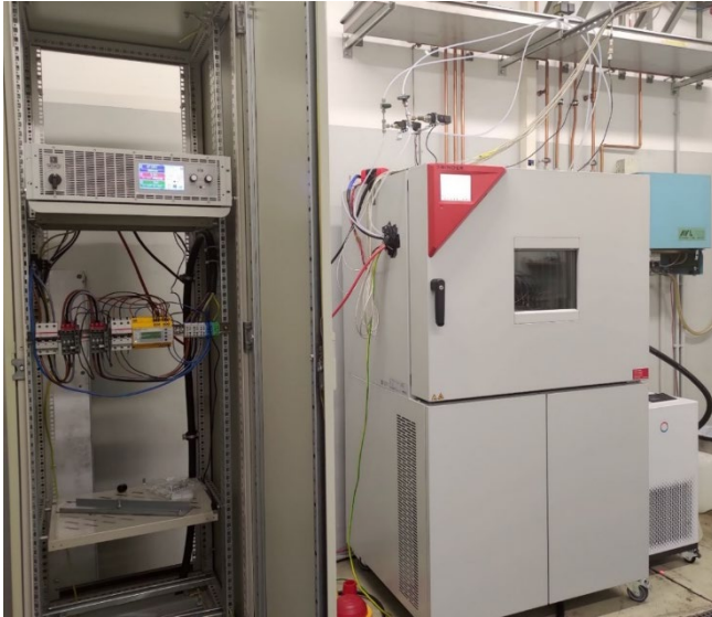
Fig. 2: Realised setup of the test bench with bidirectional laboratory power supply, temperature chamber and liquid conditioner (from left to right) (Photo: Argomotive GmbH)
